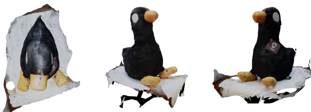
Figure 6 – Best Meshroom’s single object reconstruction attempt (attempt 3). Top model view (left), Left model view (middle), Right model view (right)
